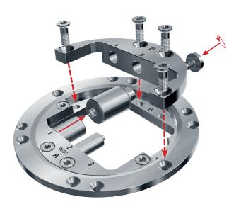
4-Screw the Pre-mill with ESPARRAGOM 5x7'5 screw. Place the flat face of the pre-mill oriented to the bottom to fix it with the clamping screw.
